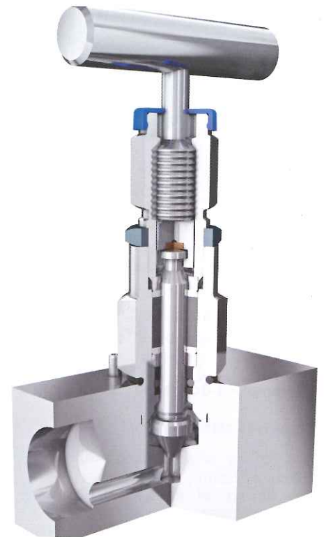
AS-Schneider E Series Needle Valves and Manifolds with Screwed Bonnet are high wear resistant and equipped with a hard coated stem thread. The non-rotating stem guarantees low actuating forces and minimum wear of the sealing elements. Pressure rating 420 bar / Class 2,500.
