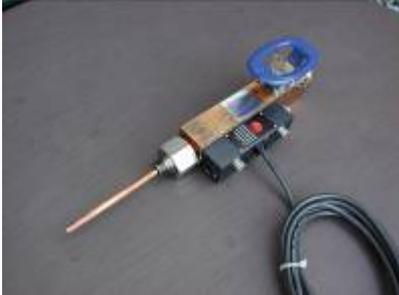
**Picture 1:** The heatable sampling probe consists of a copper block with an absorber pipe, a bolted-on heating block and an integrated ball valve.
