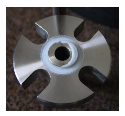
**Picture 2:** Manifolds with PTFE seal rings are clearly at a disadvantage when used at high temperatures: The plastic becomes very soft at high temperatures causing the pressure of the process medium to press it into the available cavities.
