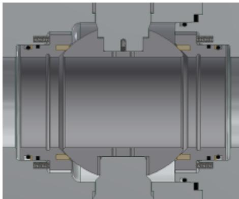
**Picture 2:** On top of that, there are ball valves with Trunnion Ball Design. In this application the balls are fixed in the direction of flow but the valve seats can move.
