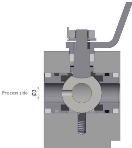
**Picture 1:** Different standards require diverse solutions. The standard SHELL MESC SPE 77/170 requires venting through a three-millimeter borehole in the ball in the direction of the process.
