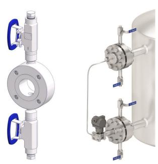
**Picture 1 & 2:** Close coupled flush rings have a direct connection to the process line and do not use impulse lines. They save users time and money while increasing their safety level.
