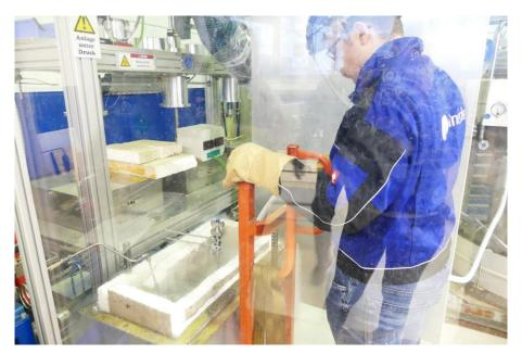
**Picture 1:** The Testing of cryogenic valves down to -196°Celsius. AS-Schneider tests its cryogenic valves in liquid nitrogen.
