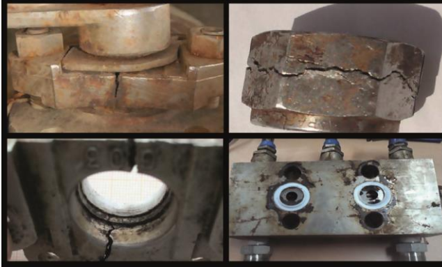
Picture 1: Corrosion cracking in pipelines
