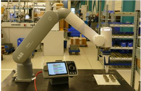
**Picture 1+2:** Collaborative robots (cobots) tested in assembly at AS-Schneider.
