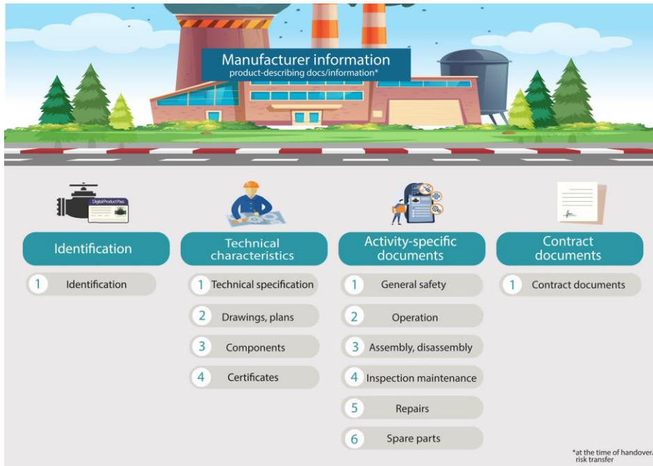
Picture 1: Classification of manufacturer's data according to VDI 2770.
