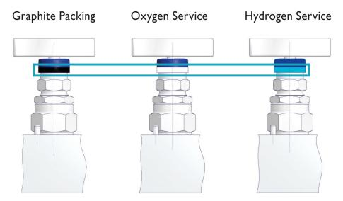
**Picture 2:** Color coding indicates graphite packing, oxygen, and hydrogen service.
