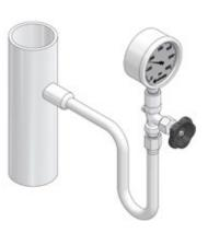
**Vertical Installation (vertical tap)**Compact Gauge Syphon and Coil Syphon
