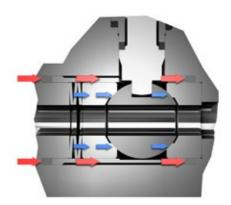
The forces needed to maintain the tightness between ball seat and valve body are only directed onto the corresponding graphite seal rings. The ball is only spring-loaded, which ensure a low, defined, minimum pressure off the balls on the ball seat. A smooth operation is the consequence.
