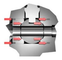
The forces required to maintain the tightness are stressing all components - even the ball and seats. The operating torque is thus very high.
