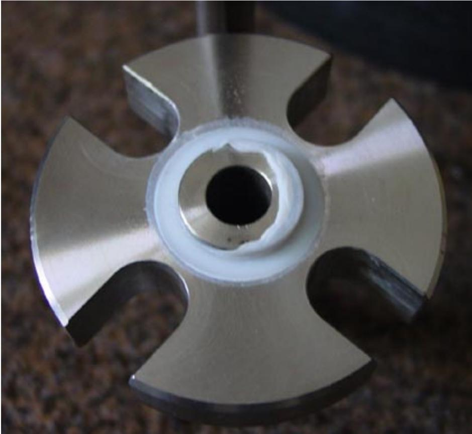
**Picture 2:** Manifolds with PTFE seal rings are clearly at a disadvantage when used at high temperatures: The plastic becomes very soft at high temperatures causing the pressure of the process medium to press it into the available cavities.
